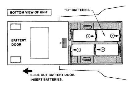
To insert batteries, slide out battery door and insert 4 "C" cell **alkaline** batteries in the order and direction shown. Replace battery door.
